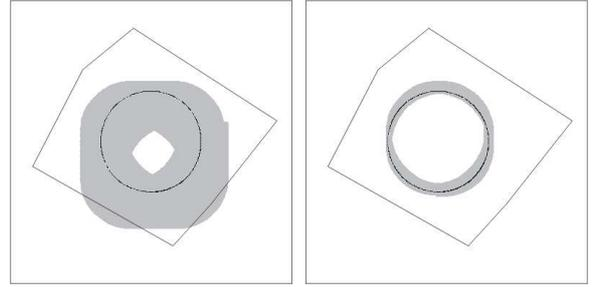
Fig. 9. Left: envelope obtained by an interval integration without using the rangefinder. Right: the information collected by the rangefinder is taken into account.
