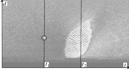
Fig. 2. A part of the waterfall collected by the portside lateral sonar of the underwater robot *Redermor* built by the GESMA (Groupe d'Etudes Sous-Marines de l'Atlantique).
