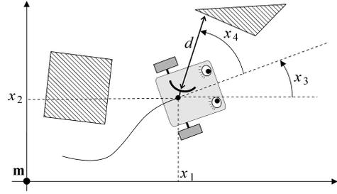
Fig. 6. The robot equipped with a rotating telemeter has to localize itself. It measures the distance  $d$  to the first obstacle. Only the location of the mark  $\mathbf{m}$  is known.
