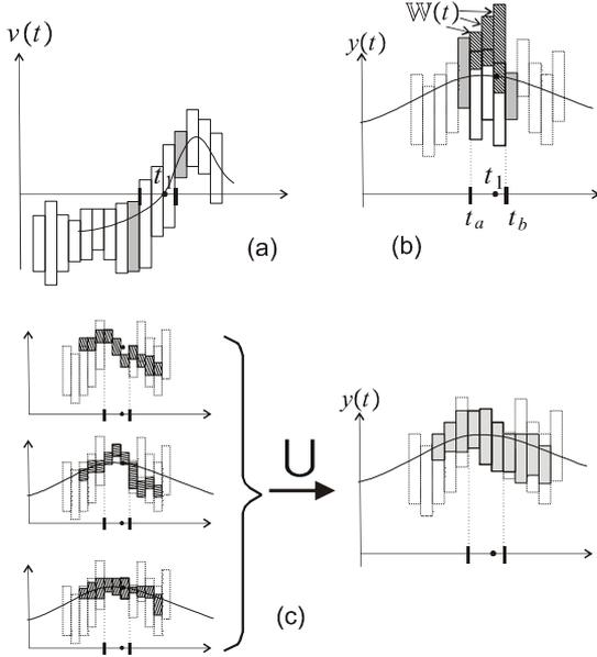
Fig. 5. Contraction of the tube  $[y]$  when we know (from the sign of  $v$ ) that a visible data has been detected.
