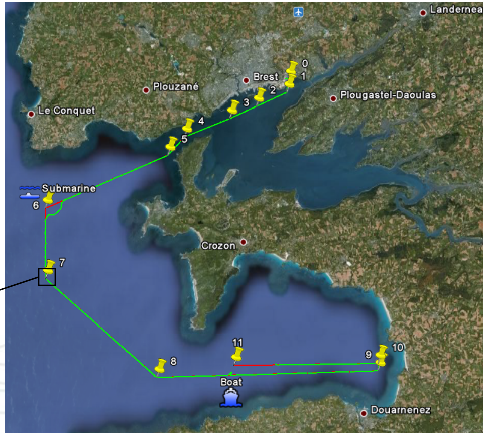
Desired Brest-Douarnenez trajectory (red lines made by yellow waypoints) and effective trajectory (green)
