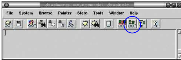
Figure 10.2: Clicking this icon opens the schematic editor interface, as illustrated by figure 8.2
