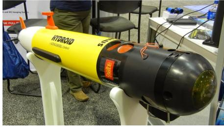
(a) Hydroid's REMUS AUV developed in collaboration.
