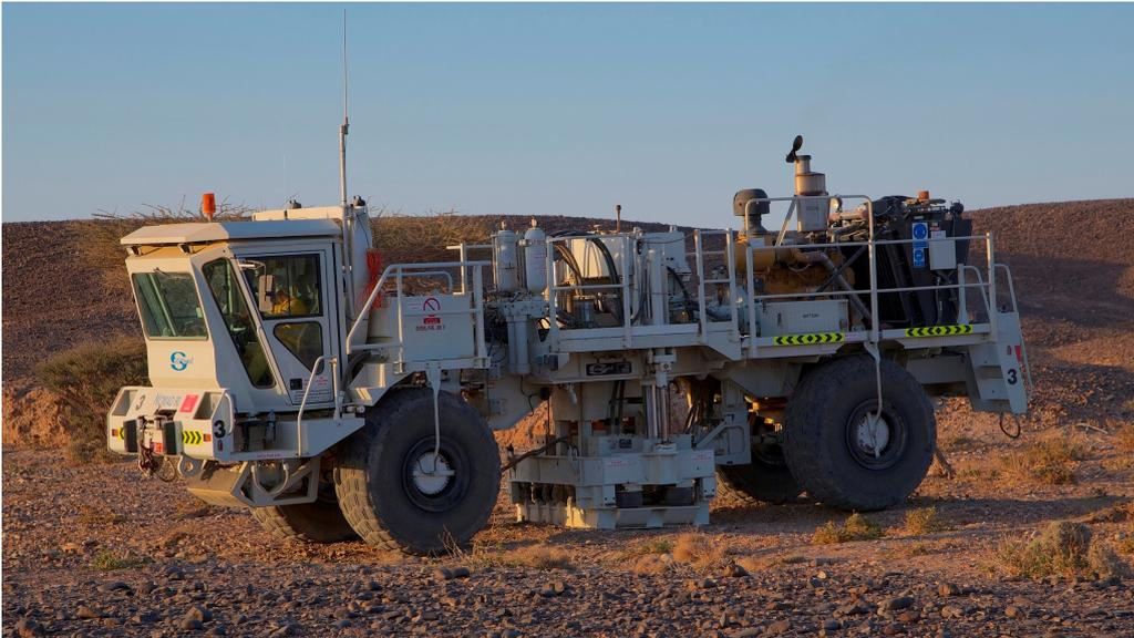
**Figure 1.7:** A land seismic vibrator: Nomad 90.
