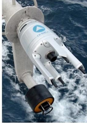
**Figure 2.6:** IXBlue Ultra-Short Baseline (GAPS) And A Modem Mounted On A Ship.
