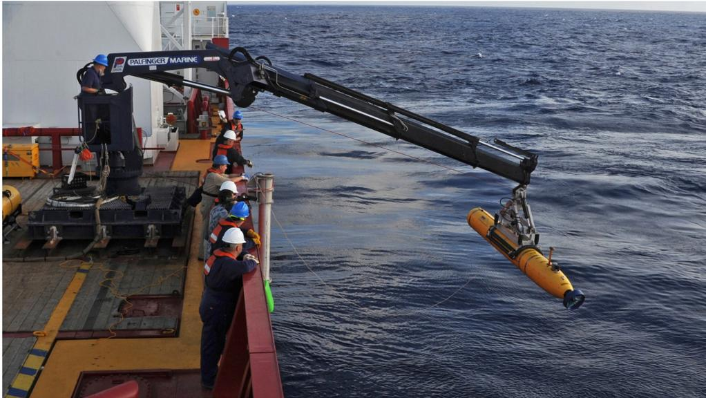
**Figure 1.1:** The U.S. Navy AUV *Artemis* (Bluefin 21') deployed from the *ADV Ocean Shield* vessel to search for the missing *MH370* at a 4000 meters depth using a side-scan sonar.
