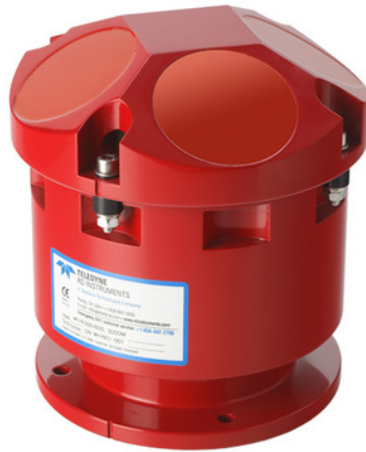
Figure 1.4: DVL. The four disks (three of which are visible here) project a high frequency acoustic signal on the seafloor and measure the received Doppler shift, allowing to measure the speed of its carrier in several directions.
