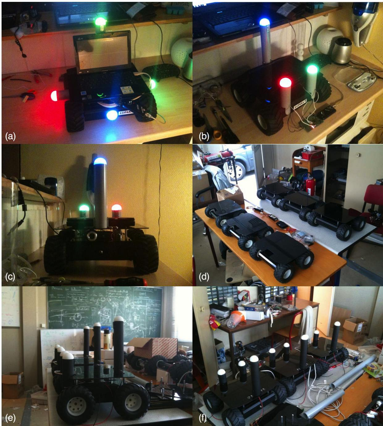
Figure B.5: (a) First prototype. (b) Second prototype. (c) Second prototype as seen by another robot. (d) The assembly line. (e) Three completed robots. (f) The robots were built identical.
