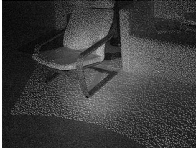
Figure A.1: Kinect's projected IR structured light
