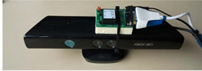
Figure A.8: The IMU is mounted on the *Kinect*.
