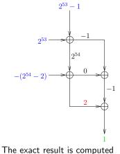
The rounding errors are computed thanks to error-free transformations.
