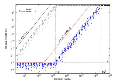
The compensated Horner algorithm is as accurate as the classic Horner algorithm performed in twice the working precision, with a final rounding.
