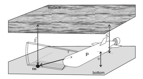
**A Loch-Doppler.** Returns the speed of the robot  $\mathbf{v}_r$  expressed in the robot frame. Also returns the altitude a of the robot  $\pm$  10cm.
