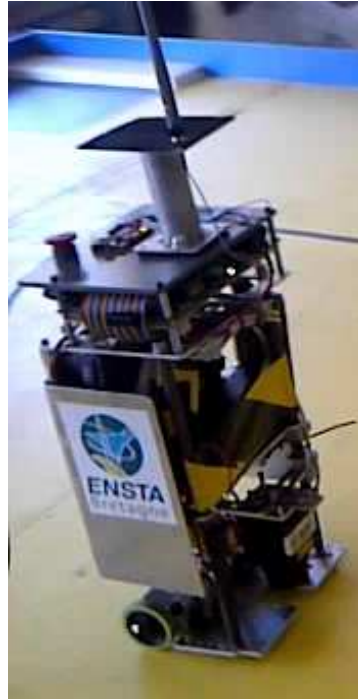
Robot equipped with a laser rangefinder and a compass.
