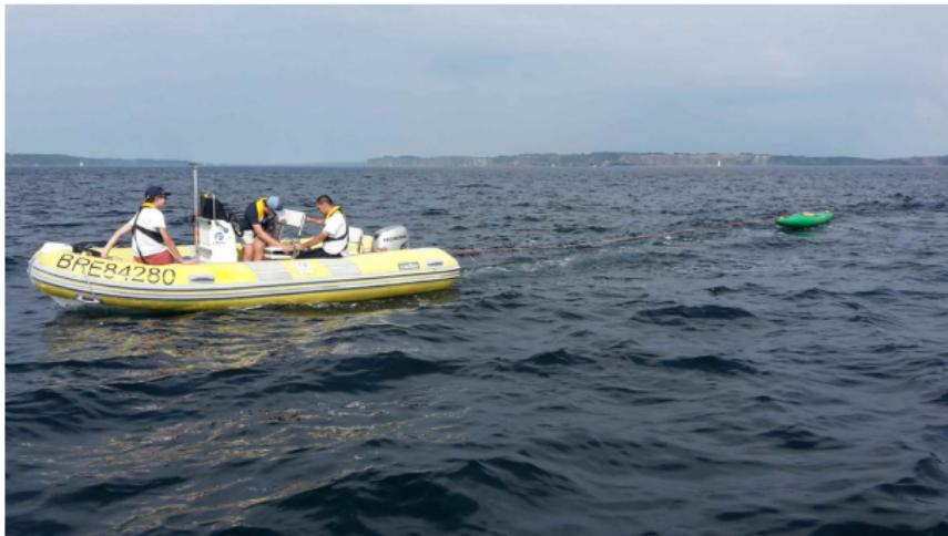
Boatbot tows a magnetometer
