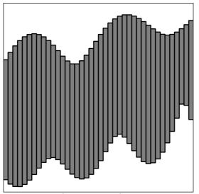
In the machine a tube can be represented by two stair functions
