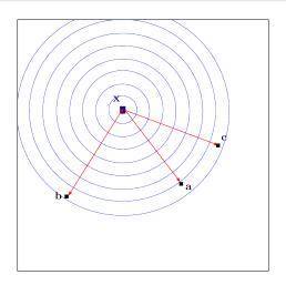
${\bf x}$  emits a sound received later by three microphones  ${\bf a},\,{\bf b}$  and  ${\bf c}$
