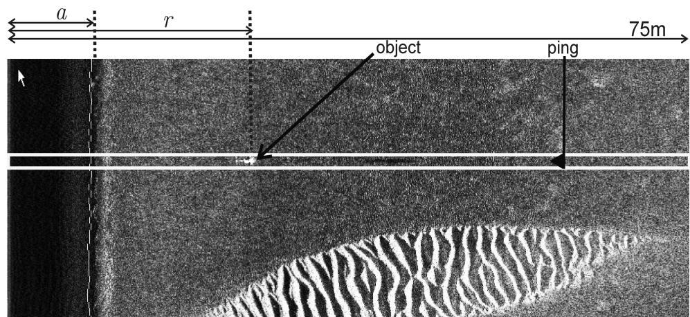
Detection of a mine using SonarPro
