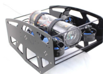
experimental platform BlueROV1, 6DOF
