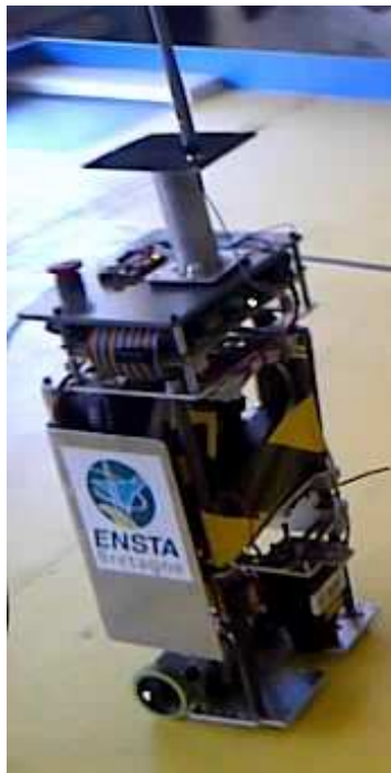
Robot equipped with a laser rangefinder and a compass.
