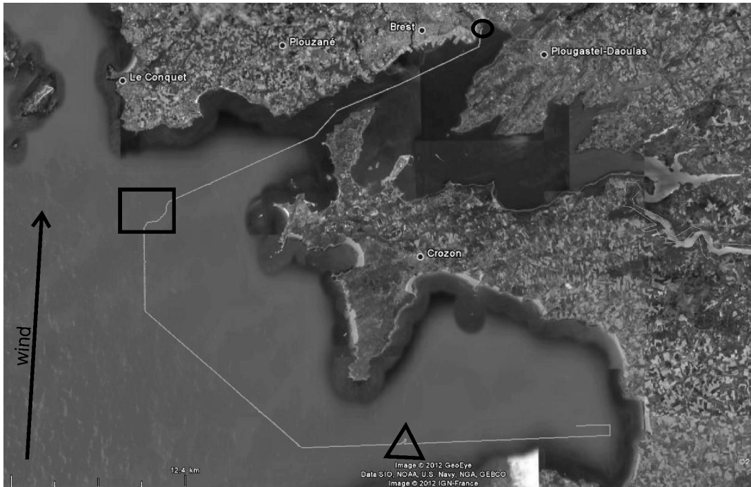
Figure 4.16: Journey from Brest to Douarnenez made by VAIMOS : (a) the robot leaves the Moulin-Blanc harbour (in the circle) ; (b) it avoids a submarine (in the square) ; (c) it avoids a cargo ship (triangle)
