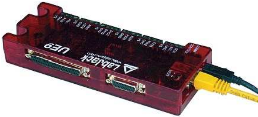
Figure 3: Le boîtier Labjack UE9
