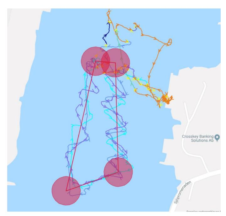
Figure 2.5: Navigation using line-follow algorithm (cyan and purple) and voter system (blue). Other colors correspond to manual mode when the boat is towed
