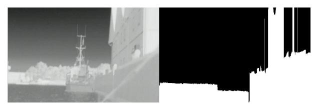
Figure 1.6: Failing situation when the bottom of the image is not water.
