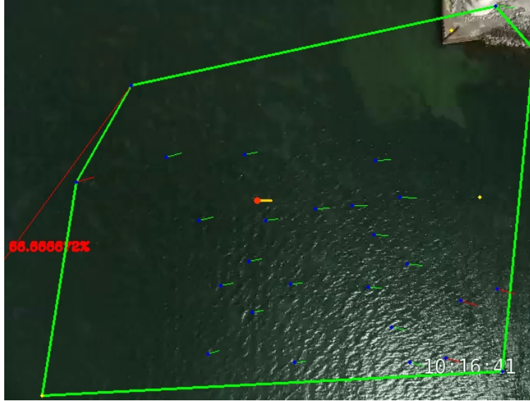
Figure 6: Optical Flow visualization on the Eiger using the down camera
