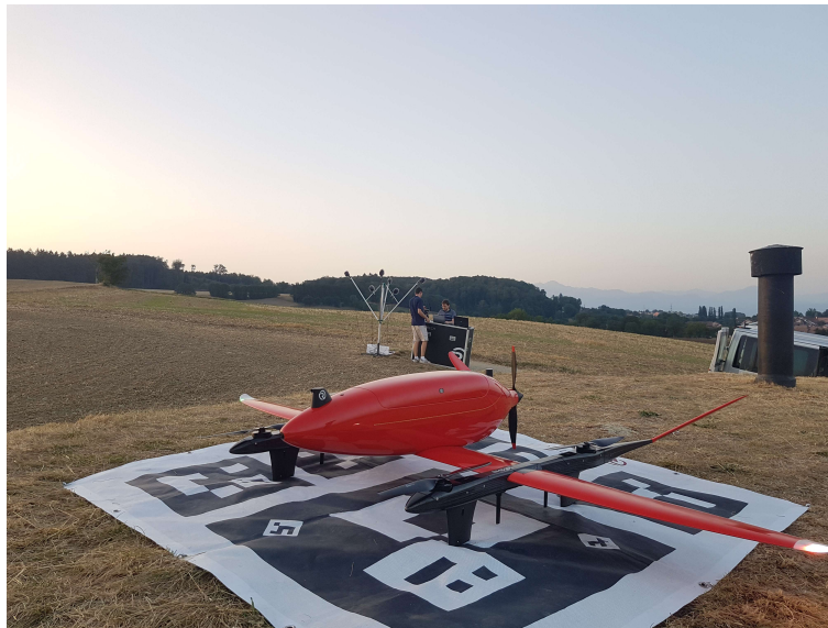
Figure 1: The Eiger on the landing pad designed for precision landing
