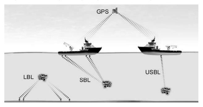
Fig 2.1 demonstrates the differences between these techniques. However, the infrastructure requirement can pose a challenge for MCM as it may not be feasible to deploy a series of transponders or a ship to aid in underwater navigation due to hazards, traffic, ice coverage or a need to be covert. Moreover, UAPS is highly dependant on the environment such as the speed of sound and the bathymetry, therefore consideration must be given when placing infrastructure.
