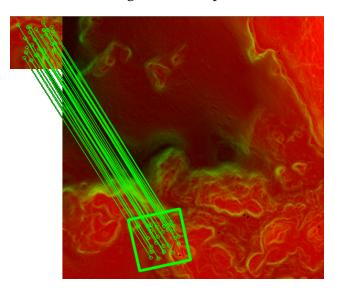
Figure 3.2 – Correlation between two sonar measures as is used in Scan Matching showing estimated displacement between the two measures
