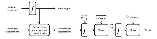
Propagation of errors is an important part of the state estimation. [11] gives a good overview of noise models. It is composed of a constant bias, a white noise and a correlated random walk. Due to this noise model, one should note that the uncertainty growth is unbounded. As a result, this method alone is unsuitable for long missions.
