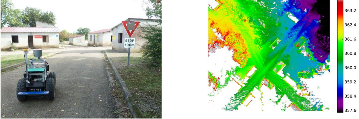
Figure 12: The ground robot with a Velodyne Lidar in the site of figure 10a, and the corresponding “atLaas” DEM (0.1m resolution).
