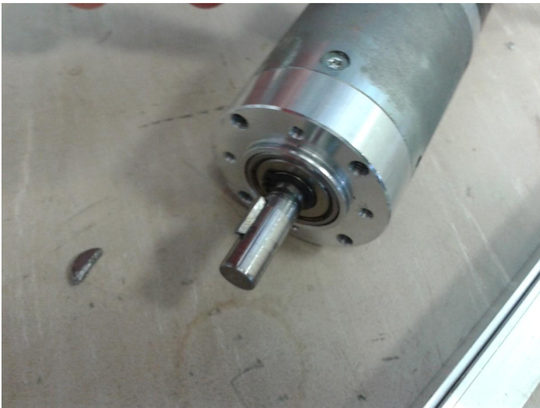
The gearbox and its new key
