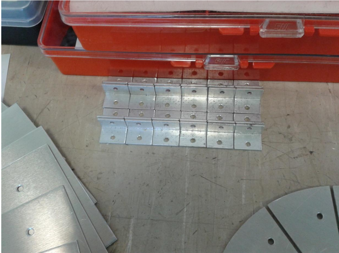
The brackets used to keep each paddle onto the disks
