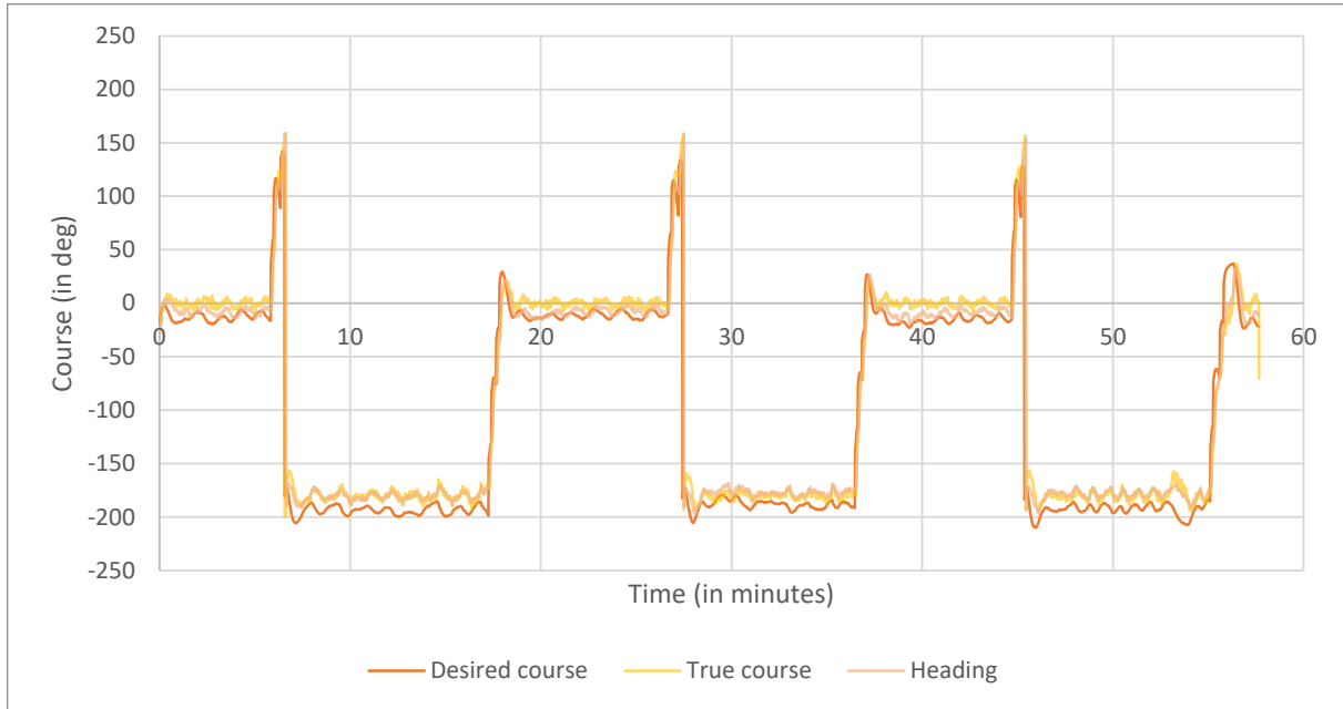
Figure 4.11: Old controller - comparison of desired course with heading and true course.
