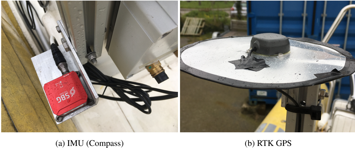
Figure 3.4: The sensors are placed on a rod beside the helm of the boat.
