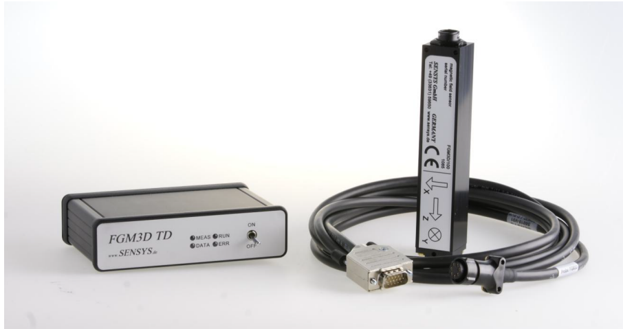
Figure 3.10: The FGM3D TD magnetometer data logging set
