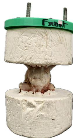
Figure 4.4: Final Preparation of Vertebrae for Testing
