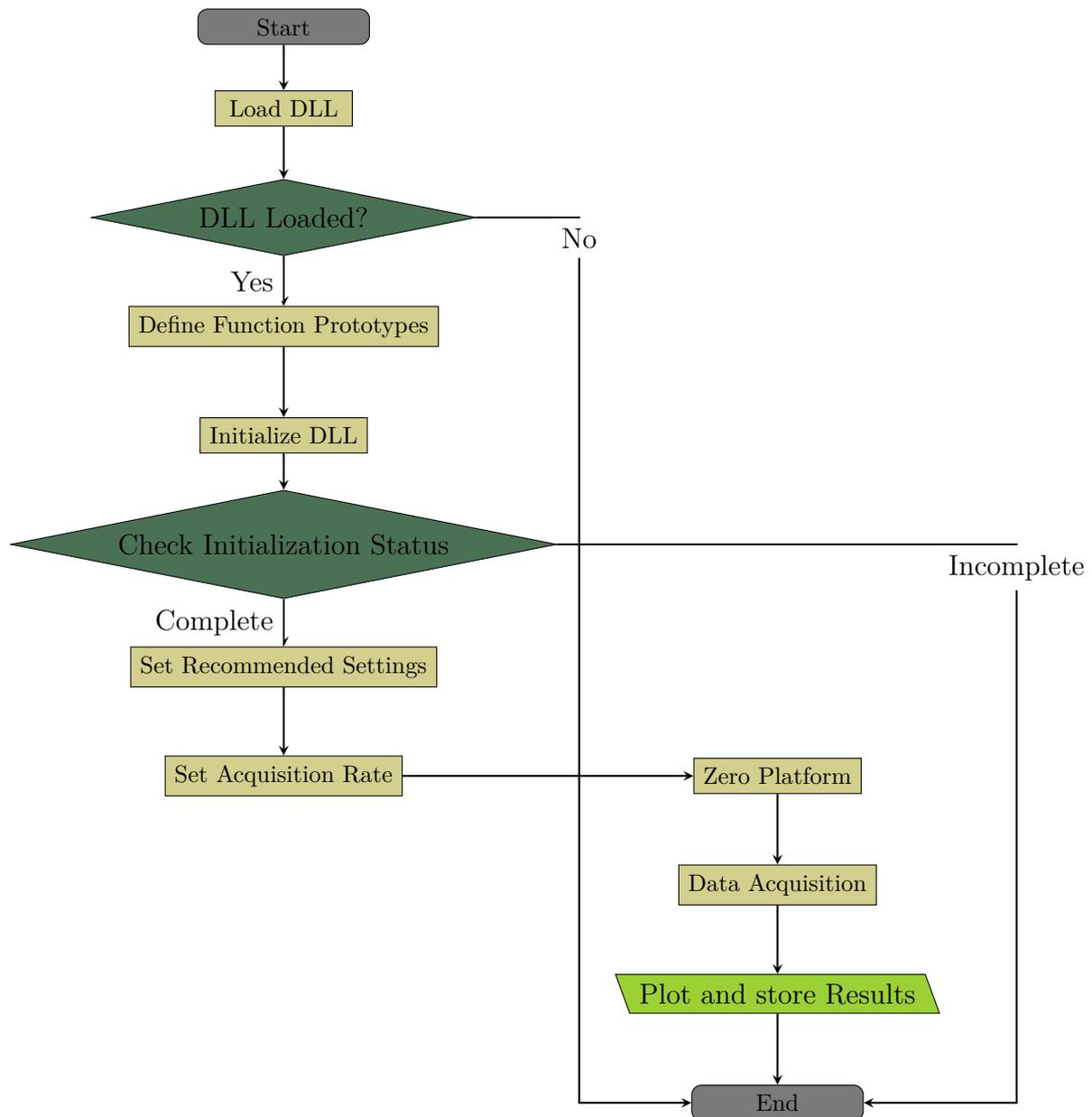
Figure 2.4: Flowchart of the Python Code for Load Cell Data Acquisition
