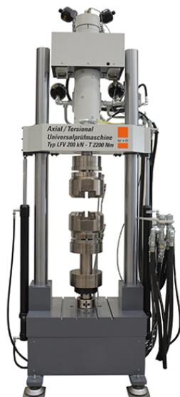
Figure 1.4: Servohydraulic axial testing system
