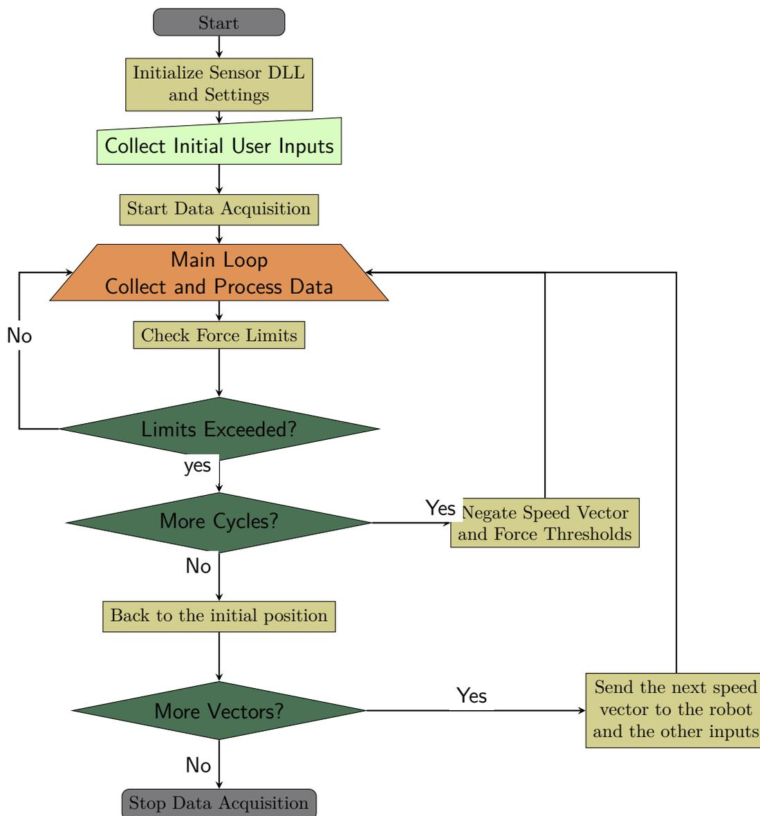
Figure 3.1: Flowchart of the Program Workflow
