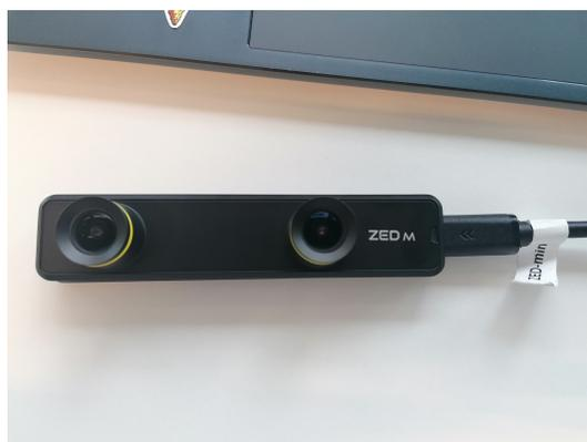
Figure 3.3: The ZED Mini stereo device
