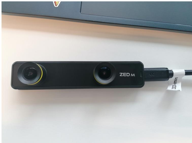
Figure 2.5: The ZED Mini stereo device
