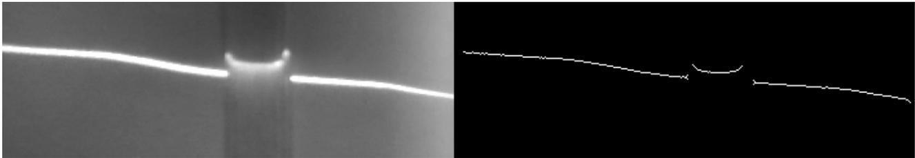
Figure 6: The skeletonization return the heart-line of a contour
