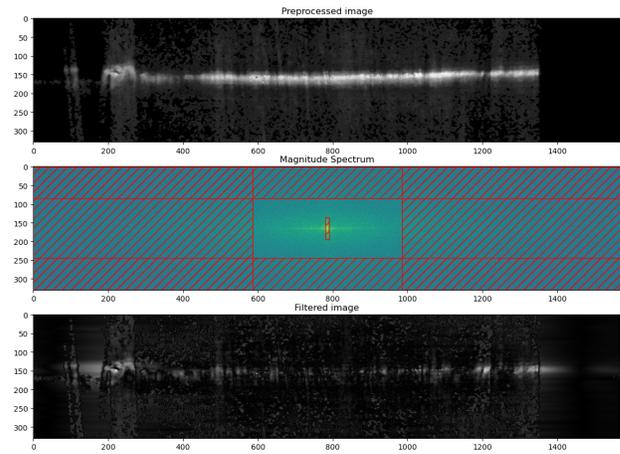
Figure 8: Fourier Transform of the image and filtering
