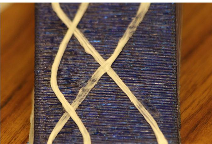
Figure 2: Variation in tow width due to uncontrolled pressure
