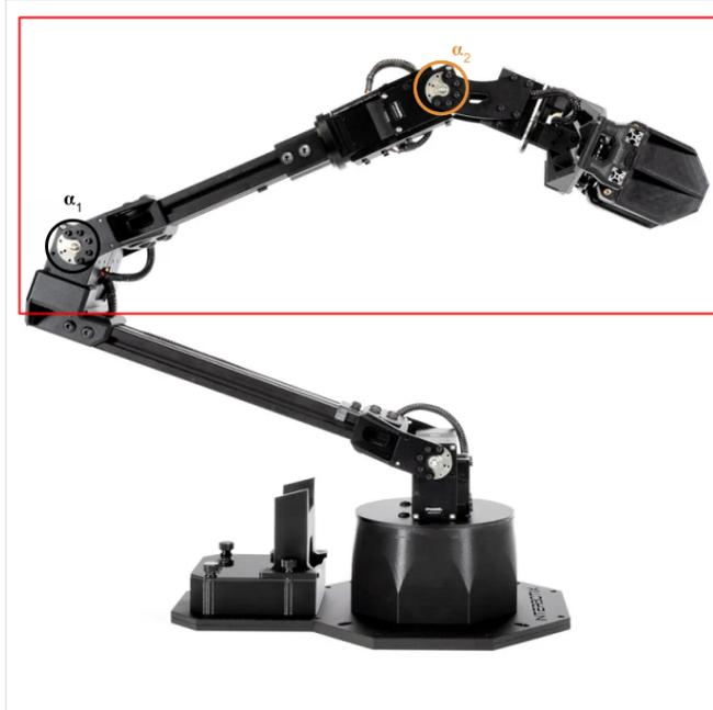
Figure 8: "Artificial" two degrees of freedom arm using the six degrees of freedom arm
