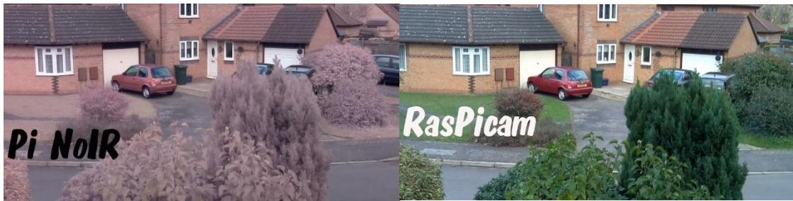
FIGURE 9 – Difference between Raspberry Pi NoIR camera (left) and regular Raspberry Pi camera (right)
