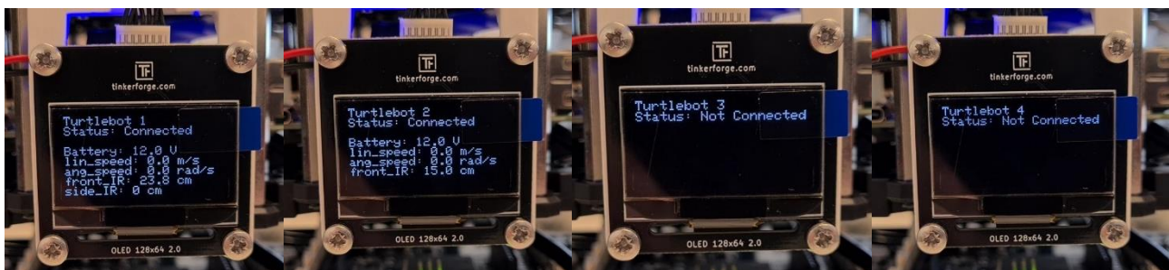
FIGURE 14 – OLED display showing the state of the different agents of the fleet
