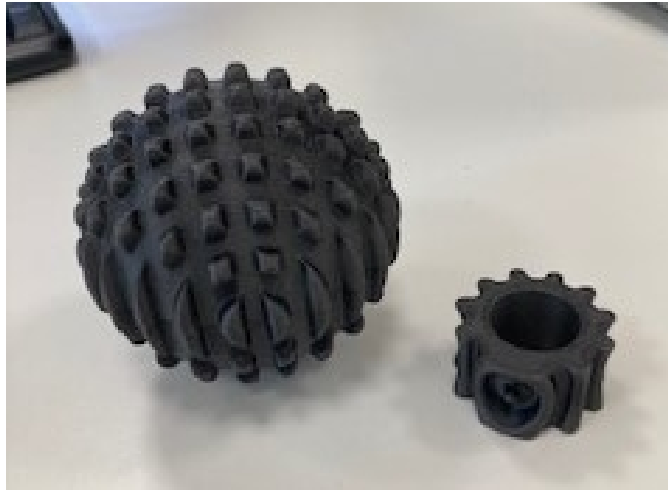
FIGURE 6 – The 3D printed sphere and monopole
