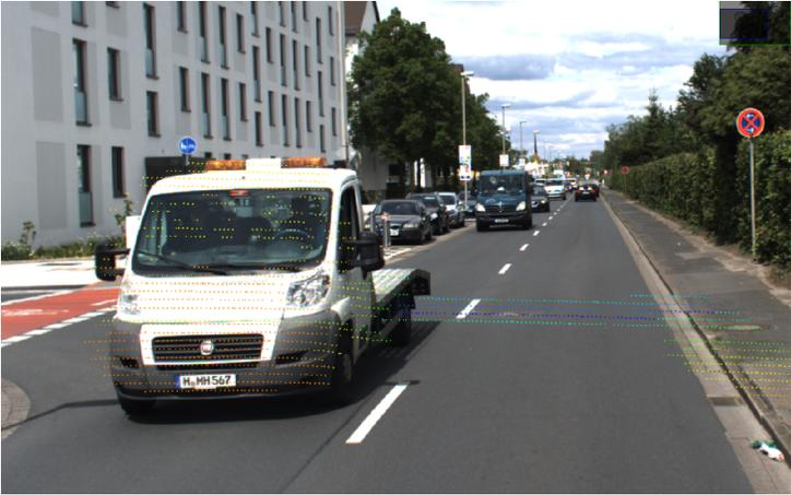
Figure 3.6: Fuse of LIDAR and camera with datas taken on the road
