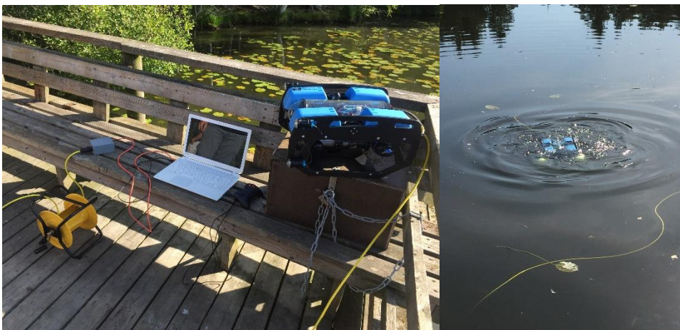
Figure 15 : Set up for lake test and BlueRov2 in water
