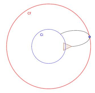
The robot is symbolized by the red triangle, Ci is the initial circle, in black there is the trajectory of the robot and Cf is the final circle, the circle that allows the robots the go back in the initial circle without leaving it.
