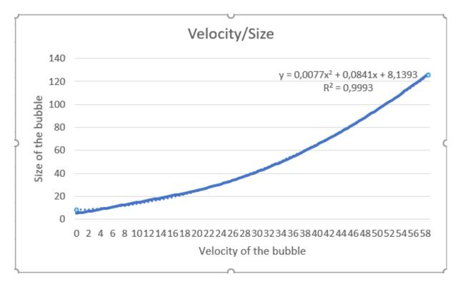
The graph represents the relation of the size of the bubble and the velocity of the bubble with a maximal speed of 60 AU, a maximal acceleration of 15AU and a maximal rotation speed of pi rad/s.
