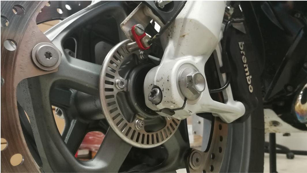
Figure 16: Speed sensor (in red) mounted on the front ABS disk.
