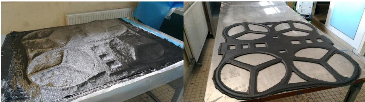
FIGURE 11 - STRUCTURE DE DRONE AVANT/APRES DECOUPAGE
