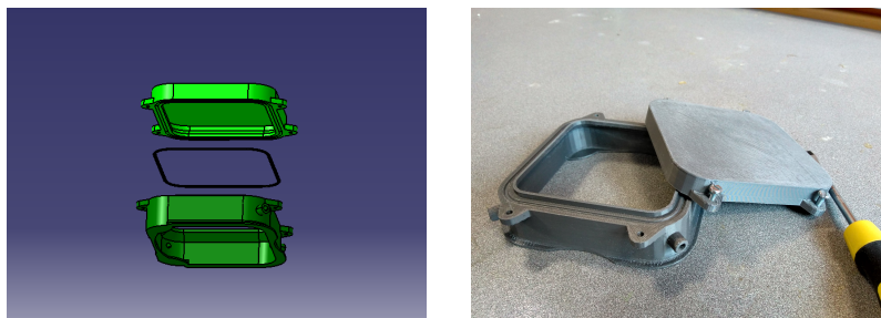
Figure 3.2: (left) 3D-Design of the cover of the boat. (right) Cover printed
