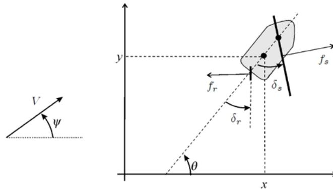
**Fig. 1.2** Notations:  $\psi$  and  $V$  define the wind orientation and speed,  $f_s$  is the force of the wind on the sail and  $\delta_s$  the angle of the sail,  $f_r$  is the force of the water on the rudder and  $\delta_r$  the rudder angle,  $\mathbf{x} = (x, y)$  and  $\theta$  are the boat position and orientation.
