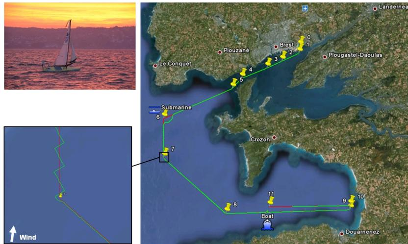
**Fig. 1.7** Brest-Douarnenez. The sailboat needed to be deviated twice: first because of a submarine coming back to Brest naval base, then because of a static boat in the sailboat trajectory. During these perturbations, the autonomous program was not changed nor stopped, the sailboat was taken by our chase motorboat. Therefore, the submarine and boat deviations illustrate the robustness of the controller, that was able to continue the mission as if nothing happened.
