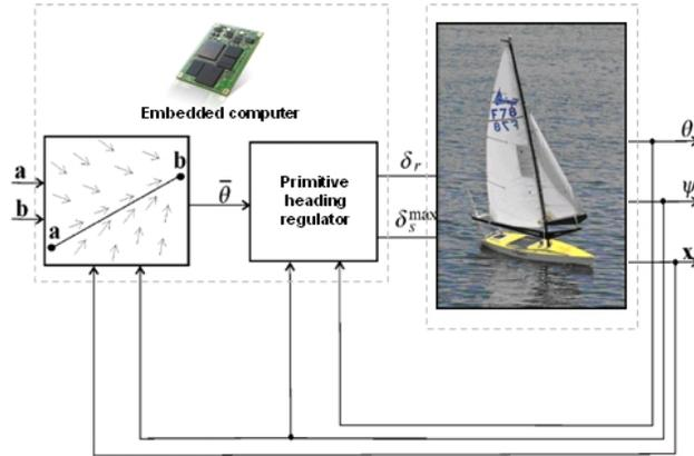
Fig. 1.3 Principle of the line following controller of VAIMOS.
