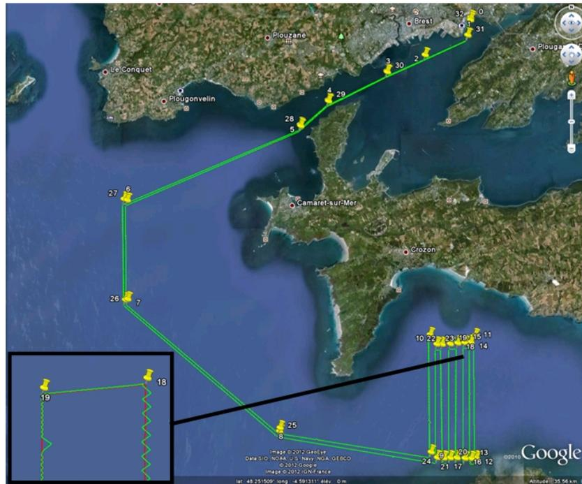
**Fig. 1.5** Simulation of *VAIMOS* going from Brest to Douarnenez. The desired trajectory (red lines made by yellow waypoints) and the effective (simulated) trajectory (green) seem to be overlapped. However, if we zoom, we see there were tacks. We see also calibration steps of the sail motor (every 2 hours) that makes the sailboat drifting during one minute.
