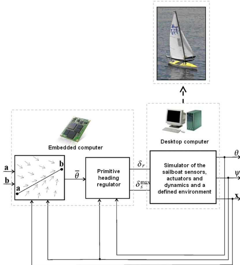
Fig. 1.4 Principle of the HIL simulator of *VAIMOS*.
