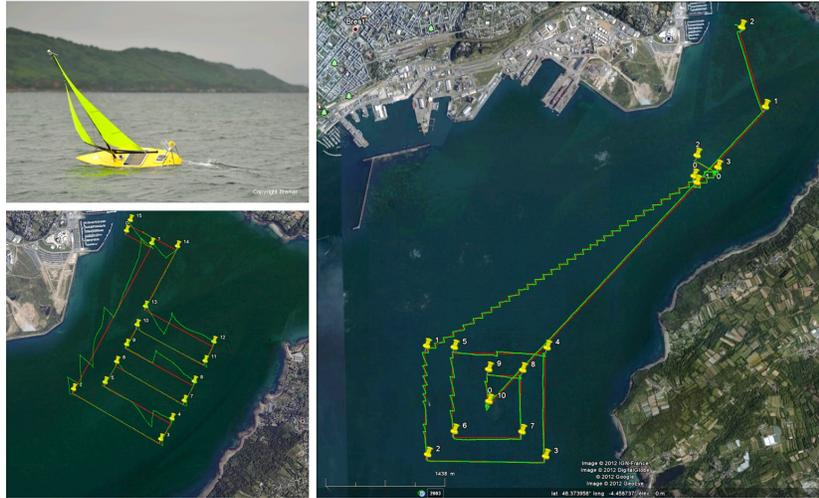
**Fig. 1.6** Tests in Brest harbor. Desired trajectory (red lines made by yellow waypoints) and effective trajectory (green). South-West wind on the left, South-West wind of around 15 kn, 27km (17 nm) in less than 5h for the right.
