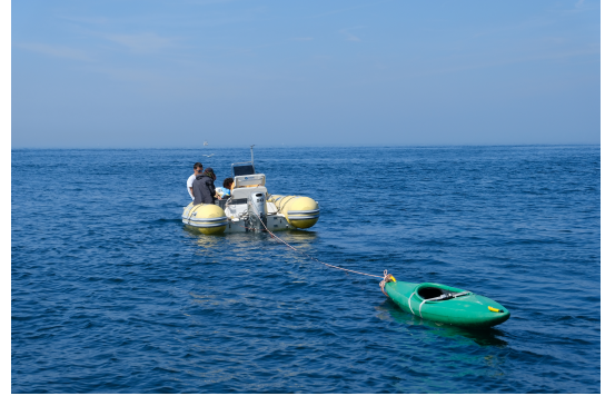
Fig. 2. Boatbot towing a magnetometer
