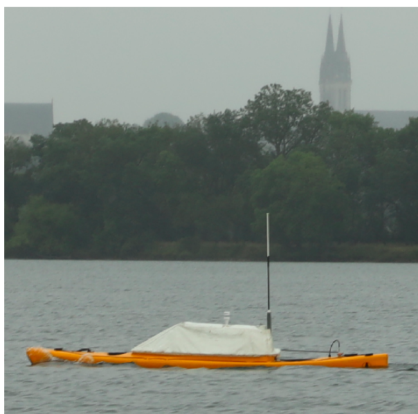
Figure 3: The autonomous kayak Mobesens moves around the buoys to collect data, Mobesens : Angers, 2022, June 22
