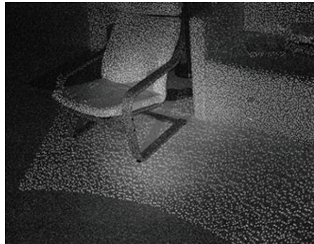
Figure 1. Kinect's projected IR structured light
