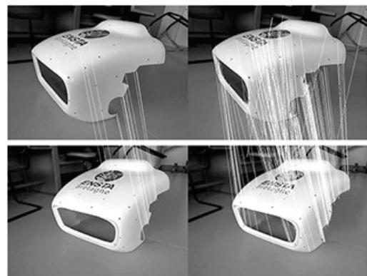
**Figure 3.** Comparison of the number of correspondences found on a mechanical prototype. SIFT is on the left and A-SIFT is on the right.
