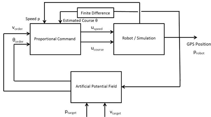
FIGURE 3.1 – Architecture of the potentials field method
