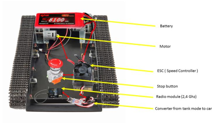
FIGURE 4.3 – Construction of the robot
