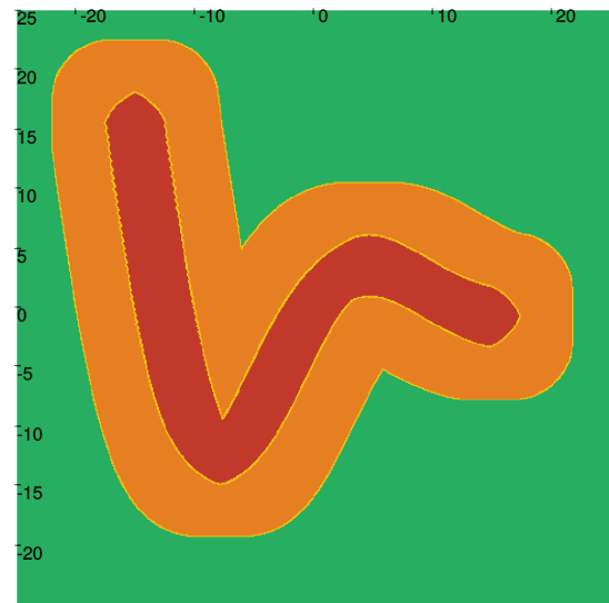
Fig. 4. Coverage of the map by the magnetometer using Thicksets
