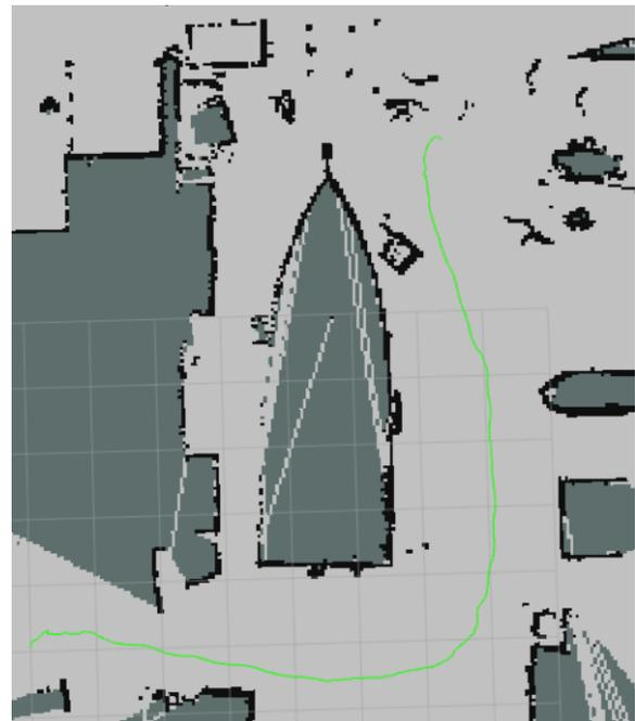
Fig. 3. Trajectory of the camera after applying scale (in green).
