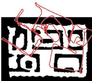
Fig. 1. Cumulative odometric errors, resulting in an unreliable path[1]
