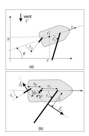
$$\begin{cases} \dot{x} &= v \cos \theta, \\ \dot{y} &= v \sin \theta - \beta V, \\ \dot{\theta} &= \omega, \\ \dot{\delta}_s &= u_1, \\ \dot{\delta}_r &= u_2, \\ \dot{v} &= \frac{f_s \sin \delta_s - f_r \sin \delta_r - \alpha_f v}{m}, \\ \dot{\omega} &= \frac{(\ell - r_s \cos \delta_s) f_s - r_r \cos \delta_r f_r - \alpha_\theta \omega}{J}, \\ f_s &= \alpha_s \left(V \cos \left(\theta + \delta_s\right) - v \sin \delta_s\right), \\ f_r &= \alpha_r v \sin \delta_r. \end{cases}$$
