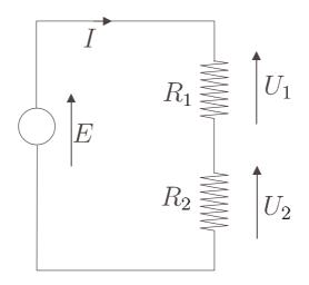
$E \in [23V, 26V], I \in [4A, 8A], U_1 \in [10V, 11V],$  $U_2 \in [14V, 17V], P \in [124W, 130W],$
