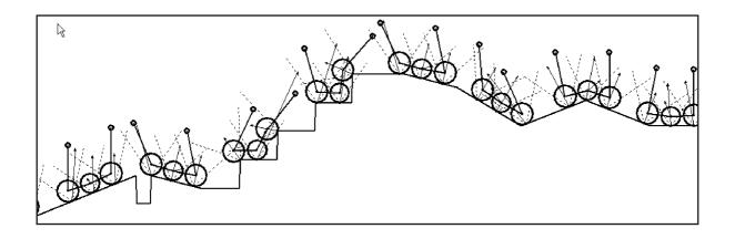
The figure below represents the robot built by the robotics team of the ENSIETA engineering school that has won the 2005 robot cup ETAS. The robot can be seen as a three-dimensional version of the robot treated above. It has been proven to be very competitive on irregular grounds but failed to cross over some compulsory obstacles (such as stairs).
