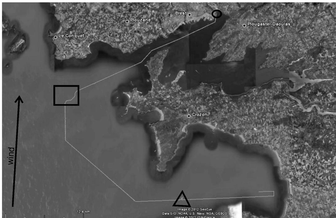
Figure 3.18: Journey from Brest to Douarnenez made by VAIMOS : (a) the robot leaves the Moulin-Blanc harbour (in the circle) ; (b) it avoids a submarine (in the square) ; (c) it avoids a cargo ship (triangle)
