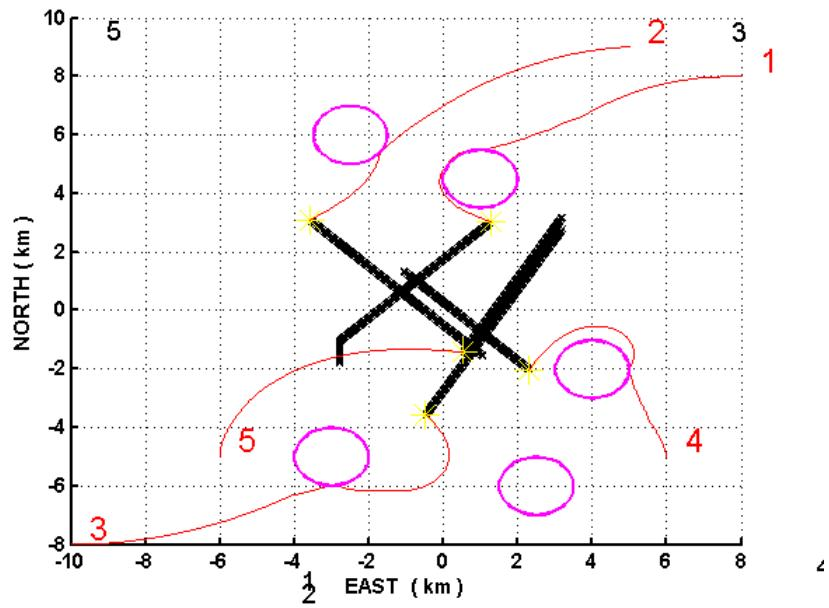
Fix obstacle collision avoidance thanks to safety bags running in parallel of a multi-agent target (re)allocation algorithm; vehicles depicted using thin red lines reach black vehicles; the obstacles are the magenta circles; red vehicles run safety bags for collision avoidance purpose
