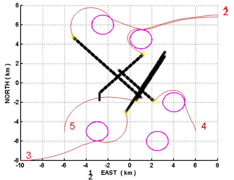
Same scenario; predefined allocation plan; no in flight reallocation allowed; demonstration of collision avoidance between two red moving vehicles (red lines top right of the figure)
