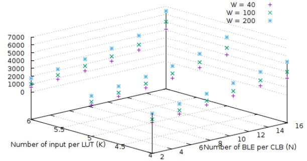
Fig. 10. Gate estimation for various architectures generated by Argen on STM 28nm FDSOI technology
