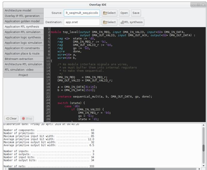
Fig. 5. Argen and user friendly DSLs for RTL descriptions: example of Piccolo experimental language.
