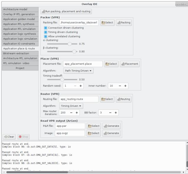
Fig. 7. Place and Route activities and virtual static timing analysis
