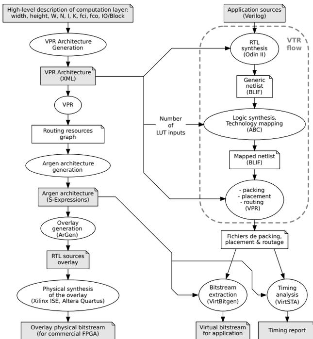
Fig. 2. Overview of ArGen tool flow
