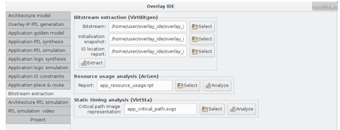
Fig. 8. Bitstream generation in Argen
