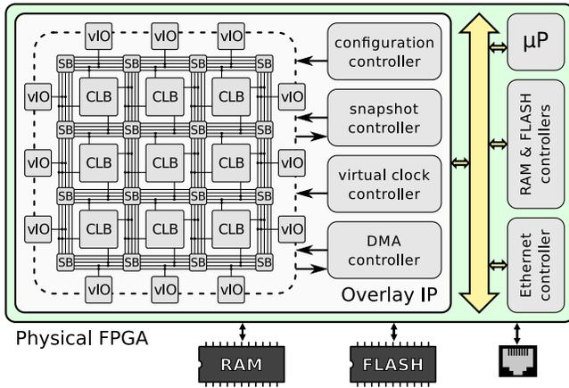
Fig. 9. Integrating an overlay in a SoC
