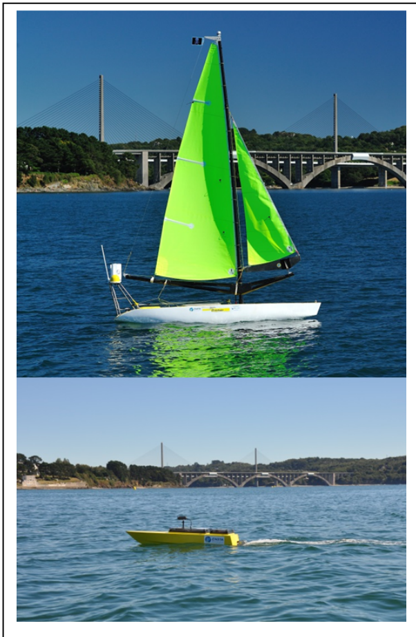
Fig. 4. ENSTA Bretagne – Ifremer team robots: VAIMOS autonomous sailboat and an autonomous motorboat built that year. VAIMOS was first at the endurance task and received the best sailboat in the open category award. The motorboat received a special prize for its success in the obstacle avoidance of known position task.
