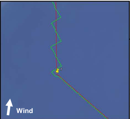
Details of a change between tack and nominal route, decided by the robot
