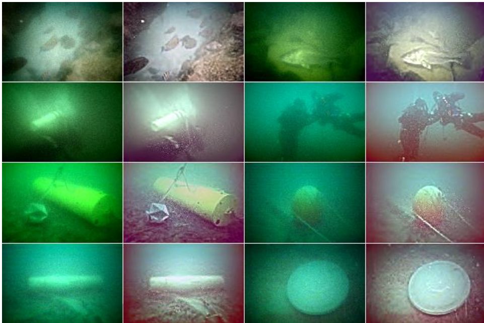
Fig. 3: Images with additional underwater noise (average blur, gaussian white noise, spot effect and color range reduced) on the left and the same images after pre-processing on the right.
